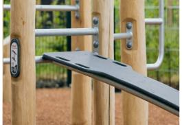
The ø414mm top plate is made from 15mm Ekogrip®, a 15mm PE plate with a 3mm top-layer of thermoplastic rubber with non-skid effect. The height is 217mm and the range of motion is +/- 90°, with a EPDM rubber stop at each end.
