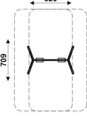
IMPACT ATTENUATING SURFACE: MAX. 42,00 m<sup>2</sup> MIN. 21,00 m<sup>2</sup>
