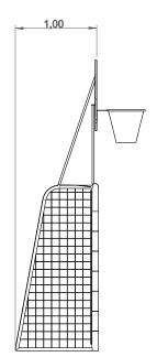
Use of the equipment under controlled conditions; Safety zone: Minimum area required by EN 1176-1,3,7
