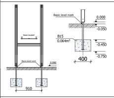
Play equipment areestablished with concreted steel foundation in equipment location. Equipment are suitable for use in two days after concreting, when the foundation are totally solid. During assambling there are not children allowed in area.
