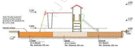
3.050 1.215 500 Thickness (According to the manufacturer's instructions for the rubber thickness in relation to the height of the fall) Base: breakstone (fr.20-40 mm); Thickness 130-250 mm
