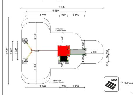
There must be in addition to 500 mm free of any obstacles in the swing direction to the rubber surface area.
