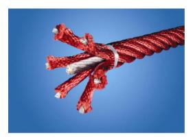
Corocord ropes with 19 mm diameter or more are special "Hercules" - type with galvanised six-stranded steel wires. Each strand is tightly wrapped with PES varn, which is melted onto each indivudual strand. The ropes are higly wear-and vandalism-resistant and can be replaced at site if needed.
