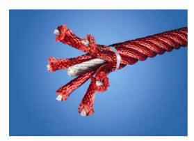
Corocord ropes with 19 mm diameter or more are special "Hercules" – type with galvanised six–stranded steel wires. Each strand is tightly wrapped with PES yarn, which is melted onto each indivudual strand. The ropes are higly wear-and vandalism-resistant and can be replaced at site if needed.
