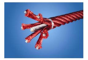
Corocord ropes with 19 mm diameter or more are special "Hercules" – type with galvanised six–stranded steel wires. Each strand is tightly wrapped with PES yarn, which is melted onto each indivudual strand. The ropes are higly wear-and vandalism-resistant and can be replaced at site if needed.
