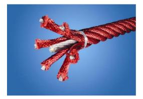
Corocord ropes with 19 mm diameter or more are special "Hercules" – type with galvanised six–stranded steel wires. Each strand is tightly wrapped with PES yarn, which is melted onto each indivudual strand. The ropes are higly wear-and vandalism-resistant and can be replaced at site if needed.
