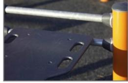
The surface is made of Ekogrip® panels, consisting of 15 mm polyethylene with a 3 mm top-layer of thermoplastic rubber. The Ekogrip® panels have a non-skid effect for comfortable and safe training at all weather circumstances.
