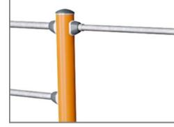
All bars intended for pull ups are made of solid, Ø32 mm x 138 cm, hot dip galvanized, S235JR steel bars. This diameter gives the right grip for everyone.
