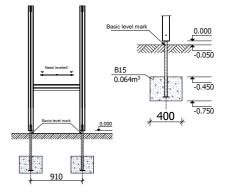
Play equipment areestablished with concreted steel foundation in equipment location. Equipment are suitable for use in two days after concreting, when the foundation are totally solid. During assambling there are not children allowed in area. Adequate temperature Snow load
