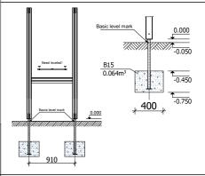
Play equipment are stablished with concreted steel foundation in equipment location. Equipment are suitable for use in two days after concreting, when the foundation are totally solid. During assambling there are not children allowed in area.
