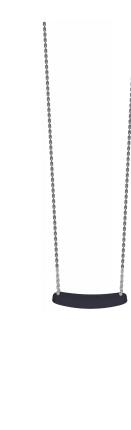
The KOMPAN swing seat is specially designed for children. It has a curved shape with a non skid surface of thermoplastic elastomers (TPE) which is moulded on an insert of polypropylene (PP) plastic. The combination of these two types of plastic gives a high value seat with a soft, user friendly surface. The seat is attached to the swing by use of Y-chains.
