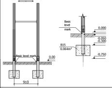
Play equipment areestablished with concreted steel foundation in equipment location. Equipment are suitable for use in two days after concreting, when the foundation are totally solid. During assambling there are not children allowed in area.
